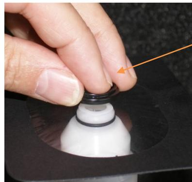
Place a film over the probe tip and hold it firm to the probe.
